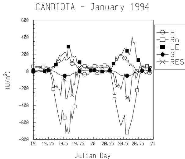
**Figure 2:** Energy flux balance. RES is the energy balance residue. Positive when directed upward.
