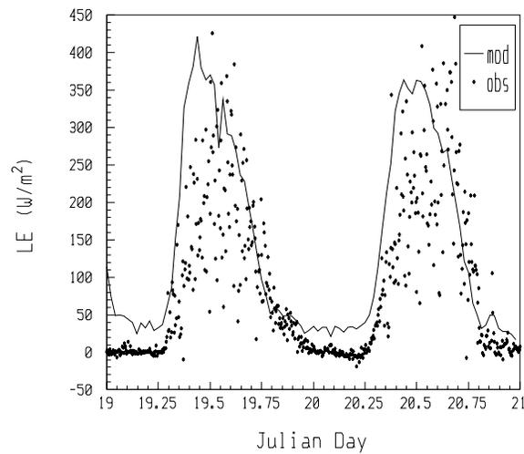
**Figure 1:** Observed and modeled (a) sensible heat flux (H); (b) latent heat flux (LE); (c) net radiation (Rn) and (d) soil energy flux at the surface (G). Positive when directed upward.
