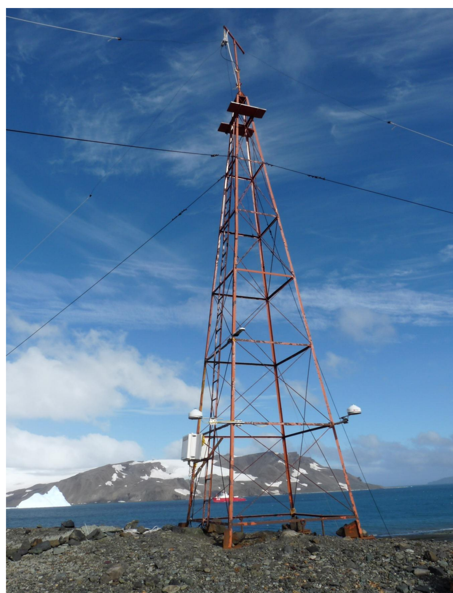
Fig. 5: Southeast view of the 12 meter South Tower instrumented with radiation sensors.
